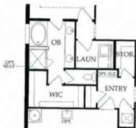
Tub Upgrade @ Owner's Bath
